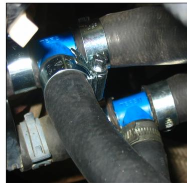
Fit tees into the hoses and run two new coolant lines to the heat exchanger.
