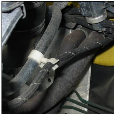
Locate the hoses that run through the bulkhead to the internal heater matrix.
