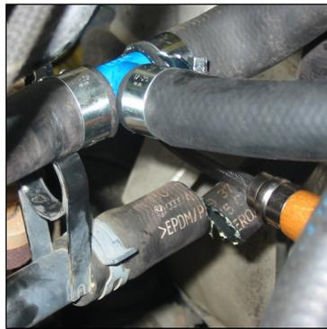
Cut into both hoses, collect any coolant that escapes in a container.
